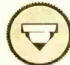
Shaft position in knob requiring 3/32" flat.
