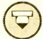
Shaft position in knob requiring 1/32" flat.
